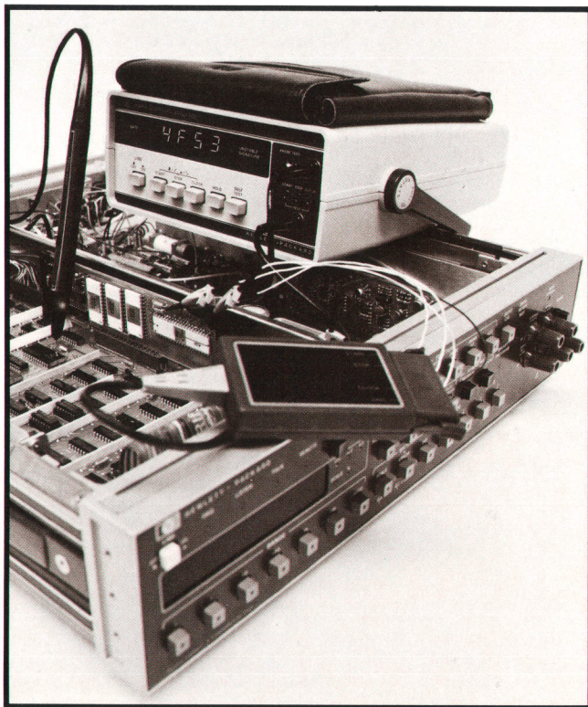
Fig. 7. Model 3455A System Voltmeter is the first HP instrument designed for troubleshooting with the 5004A Signature Analyzer.
